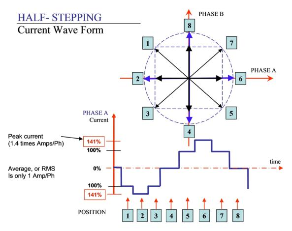
The position versus time graph just above, plots only the A Phase, following the eight different steps the motor will make. Current is changing with each position. Recall that a negative in electronics simply means reverse direction of current flow.
