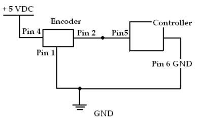
Figure 17: Encoder Pin Connection Schematic
