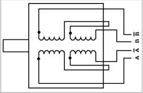
Figure 22: 8 Lead Wire Series Connection
