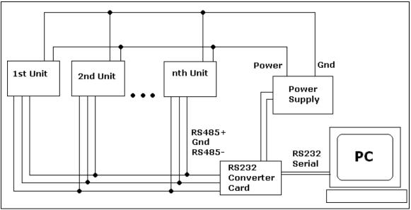
Figure 12: Connection using RS232 Converter Card
