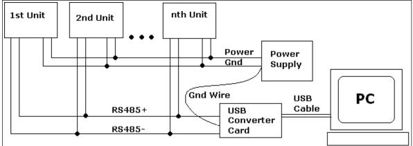
Figure 13: Connection using USB485Converter Card
