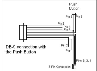
Figure 15: Push Button Schematic
