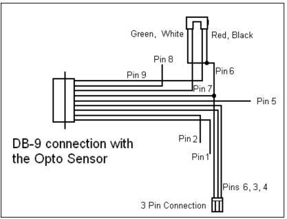
*Figure 16: Opto Sensor Connection Schematic*
