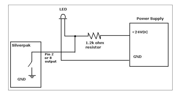
Upon entering command /1J0R, both pins 2 & 8 will output 1 Amps. The 1.2k ohm resistor will limit the current to 20 milliamps into the LED. Select any ohm value to limit your current based on the device that is connected to the output.
