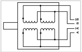
Figure 21: 8 Lead Wire Parallel Connection
