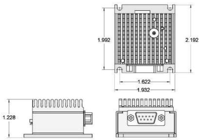
Figure 1: Dimensions Diagram
