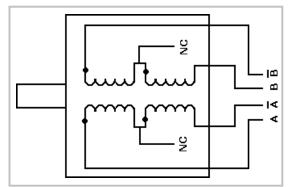
Figure 20: 6 Lead Wire Full Winding Connection
