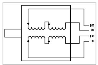
Figure 18: 4 Lead Wire Motor Connection
