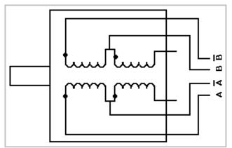
Figure 19: 6 Lead Wire Half Winding Connection
