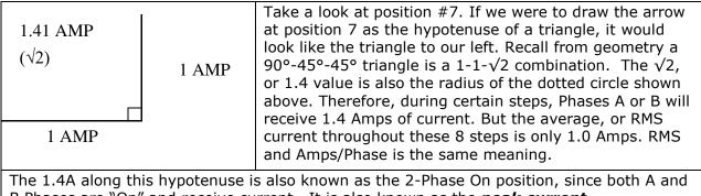
B Phases are "On" and receive current. It is also known as the **peak current.**
